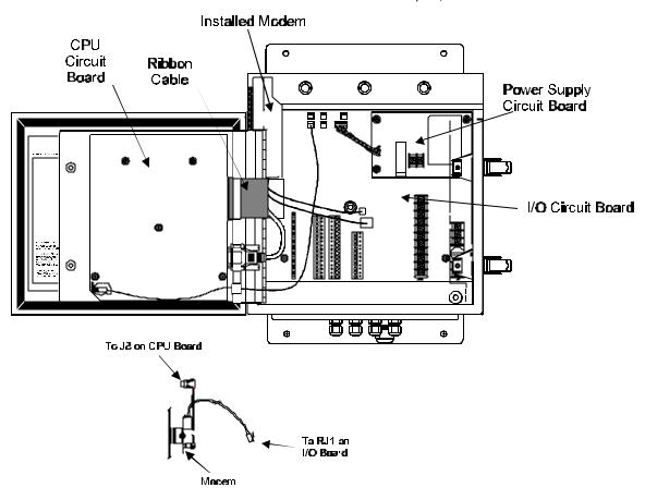
Figure 3-11: Modem Location and Connections
